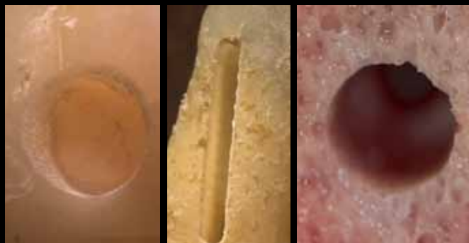
Samples of easily achievable scanning patterns in hard tissue drilling and cutting.
